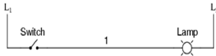
Fig 3.7 : A simple ladder diagram showing a lamp that is controlled by a switch
